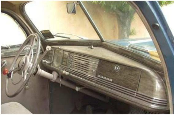
Nevertheless, the Dodge was built with entirely modern creature comforts. It features dual electric windshield wipers, sealed beam lamps, floating power, hydraulic brakes, telescopic shock absorbers, a column-shifted, synchronized transmission, tinted glass, a chromed horn ring, and a host of other innovations.
